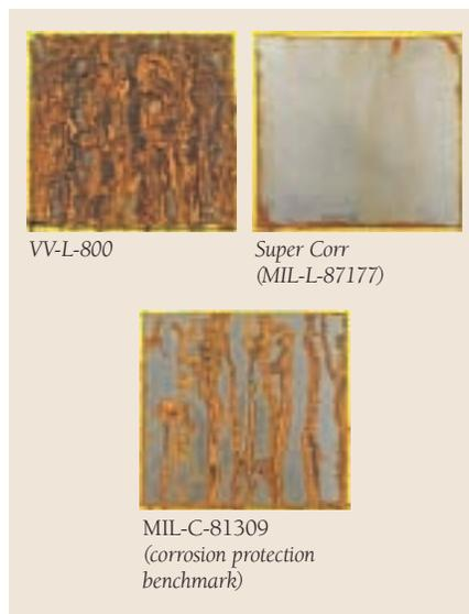
FIGURE 2: A second round of tests determined that the lubricating and corrosion protection properties of Super Corr were superior to the product being used by the P-3 squadron at NADEP Jacksonville.
