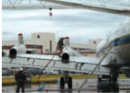
A U.S. Customs Service P-3 going its 28-day wash at the wash rack in Jacksonville. Notice the powerful water stream used to remove contaminants from the skin and exposed components.
